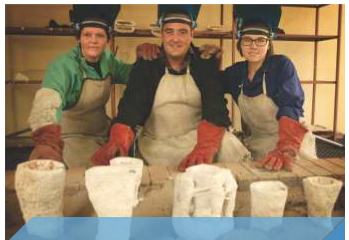
The sandpit with thick investing moulds ready to receive the bronze, from left: Ms Elsabé Dalton, James Shaw, and Marelize van der Merwe, third-year students.
