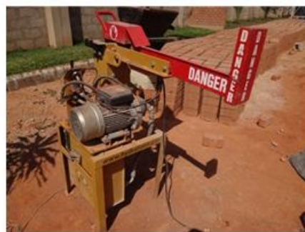
Fig. 4: CEB machine and products Source: Author Archive. Nov 2017
